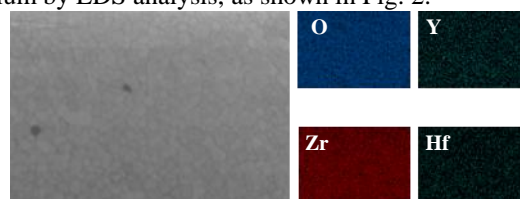
Fig. 2 Image and X-ray maps of ultra-thin 3YSZ substrate by EDS.
